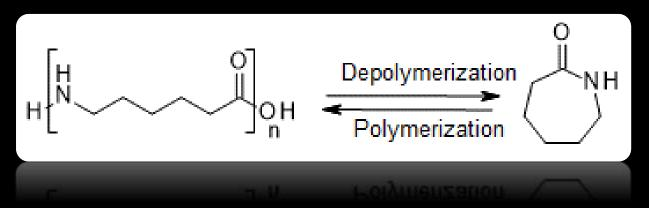
Recycling of PA6 is highly attractive as it is a polymer with a high carbon footprint (6,7t CO2 /t polymer in Europe)
